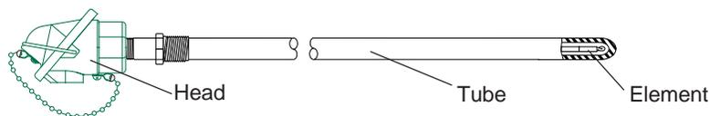
The protection tube, head and element are discrete components. The element is manufactured with individual conductors welded together at the tip. Element wires are separated by ceramic insulators. The protection tube can be thin wall tubing, schedule 40 pipe, ceramic or cast iron. Cold end termination is usually with a head and terminal block assembly.
