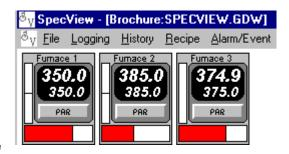
SpecView is configured using either menus or the toolbar: Tool tips identify what the function is of each tool - just move your mouse to the tool.
