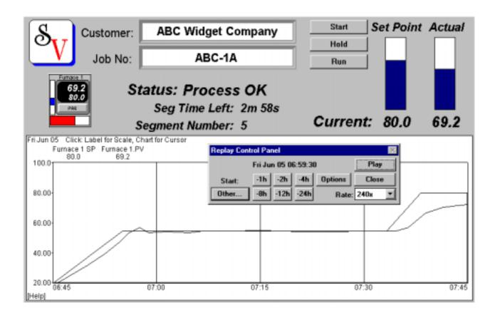
Note that **all** logged data is replayed, not just the trend chart. Numeric values, bar charts and text strings all replay. The best analogy is a video recording of the screen, replayed with an adjustable fast forward!
