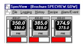
The auto detected instruments have names assigned by SpecView. These may be changed to logical names for clear identification.
