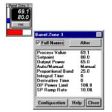
Clicking the "PAR" button displays the parameter list for the instrument.
