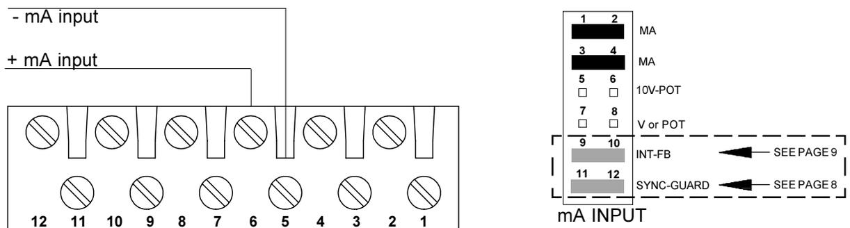
**MA INPUT: COMMON TO TERMINAL 5, + INPUT TO TERMINAL 6**
