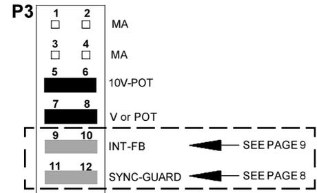
**Figure 9.** Jumper positions for Voltage inputs.
