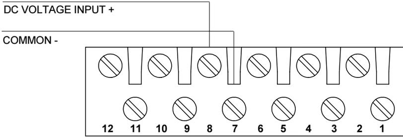
**Figure 8.** Connections for a voltage command signal.
