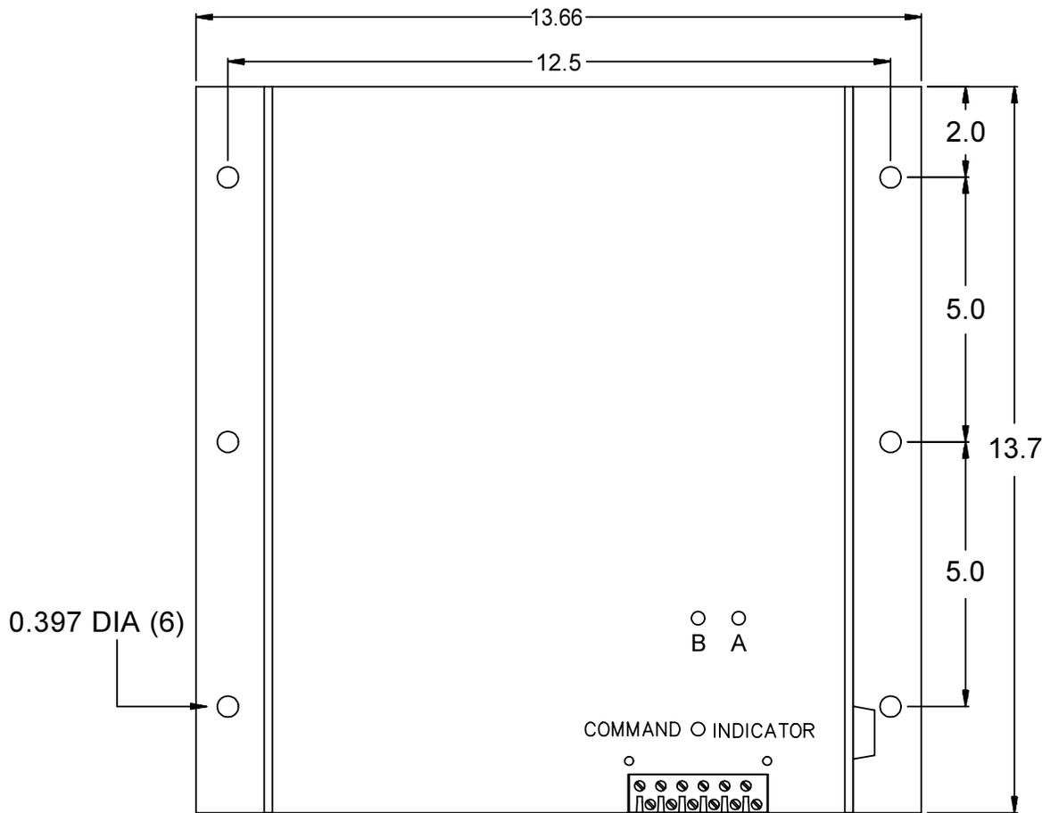
**Figure 2.** Mounting dimensions, Model 3037, 240 to 425 Amps.
