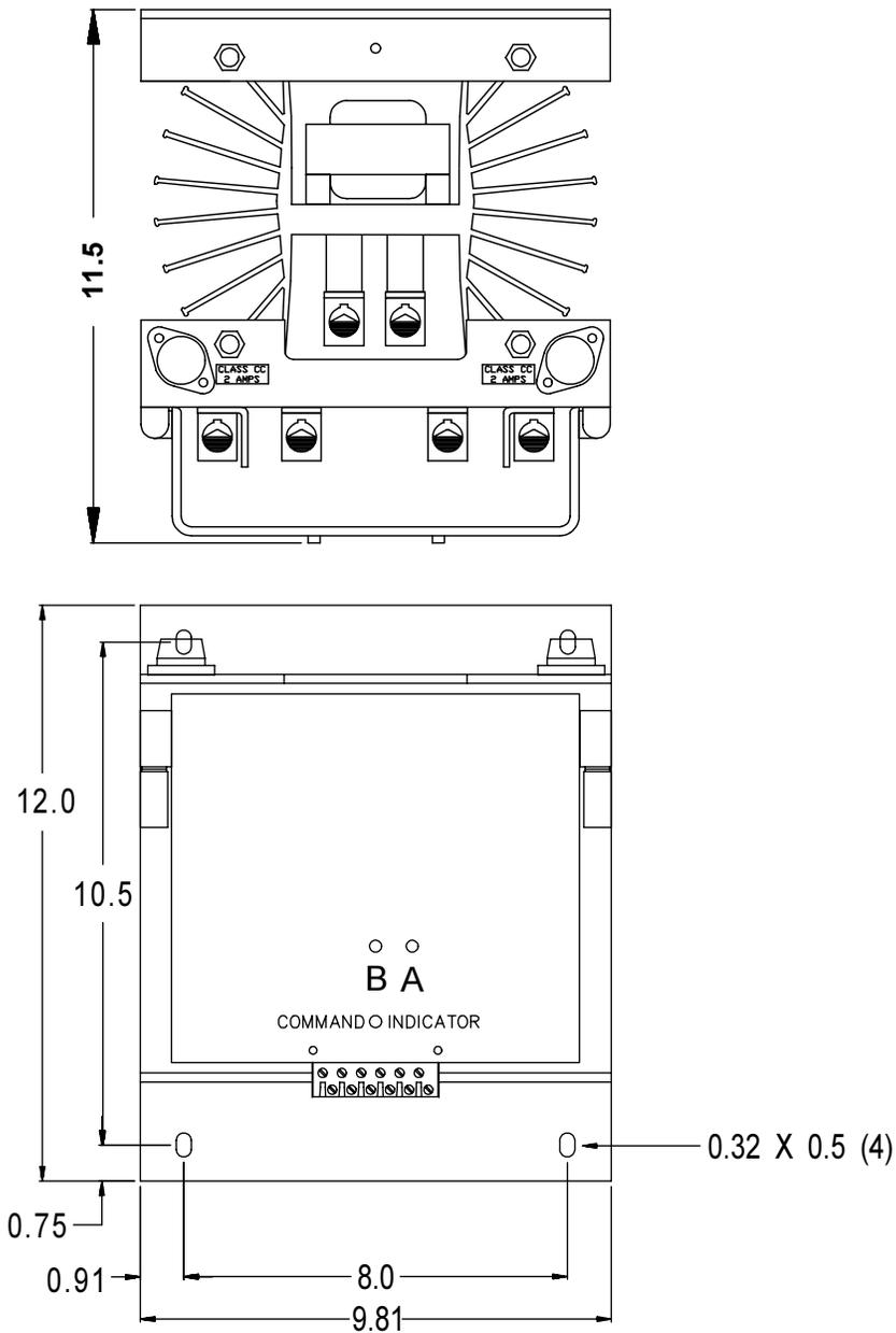
**Figure 1.** Mounting dimensions, Model 3037, 85, 145 and 175 Amps
