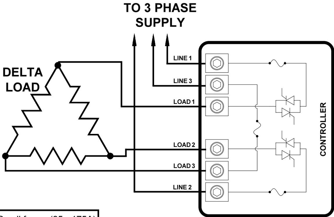
**NOTE:** Small frame (85 - 175A) has one lug per connection. Large frame (240 - 425A) has two lugs per connection.
