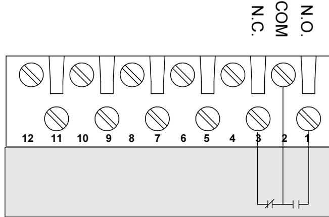
Figure 3. Connections for shorted SCR detection relay.
