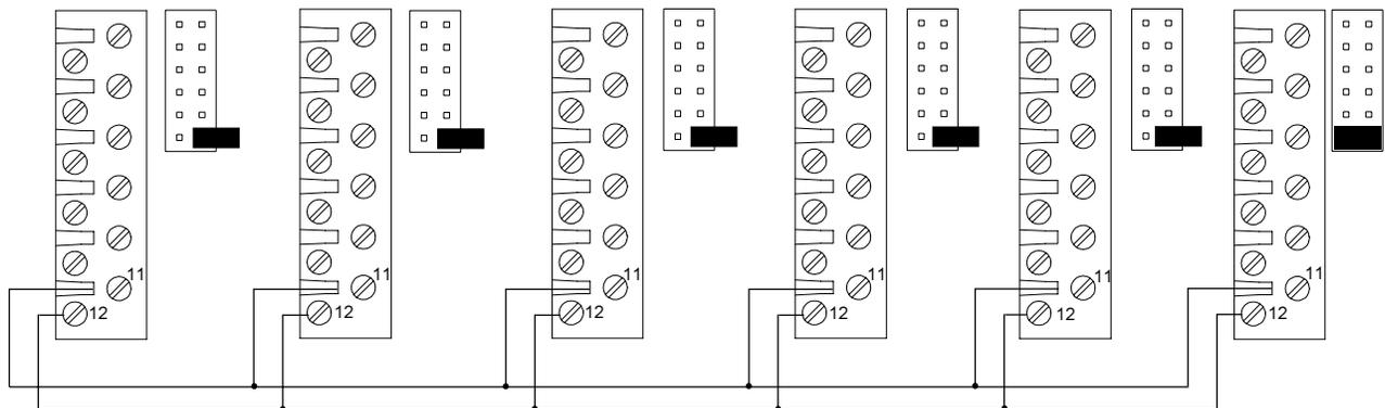
Figure 4. Connecting units together for sync guard.
